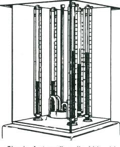
Simple, fast reading...liquid level in tubes show braking ability of each wheel with a fifth tube for total braking effort...detect low, unequal or unsafe braking conditions at a glance.
