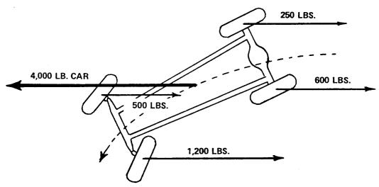
The desired direction of travel is shown by the large arrow. Excessive brake energy on the left front wheel tends to pull the front end of the car to the left, while excessive brake energy on the left rear wheel tends to make the rear end slip to the right, still further aggravating the twisting motion or skid of the car.
