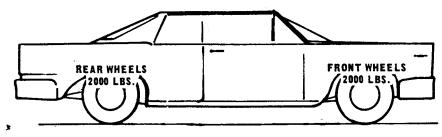
The same car on a quick stop shows one sixth of total car weight (667 lbs.) transferred from the rear to the front wheels, so that the weight carried would be:
