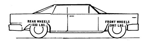
Now if you will refer back to our 4000 lb. car with four equal brakes applying 750 lbs. pressure each, you will see that when it makes a quick stop with full brake power applied, we are using 1500 lbs. of effort on the rear wheels to stop 1333 lbs. of weight, or a brake energy of 112.5% — more than enough to skid the rear wheels on the best pavement we know. On the front wheels we have the same brake energy used to stop 2667 lbs. or a brake energy of about 56% — just half as much.
